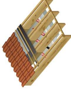
Over rafters only ventilated
