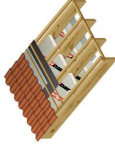
Between and under rafters ventilated
