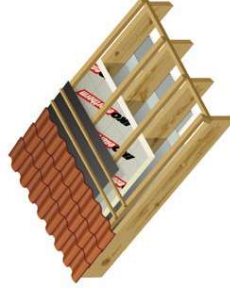
Over rafters only unventilated
