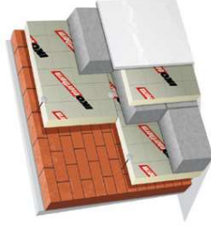
Partial fill with insulated plasterboard
